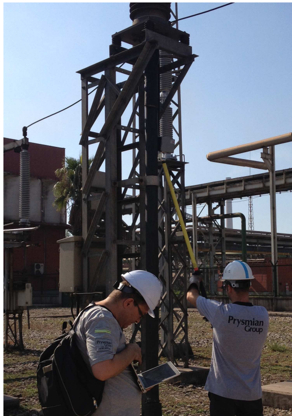
Figure 7 – Pry-Cam™ during a field measurement.
