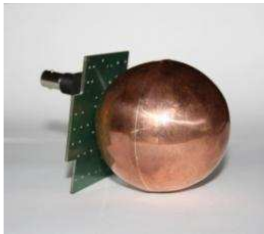
Figure 8 – The patented electric field sensor.
