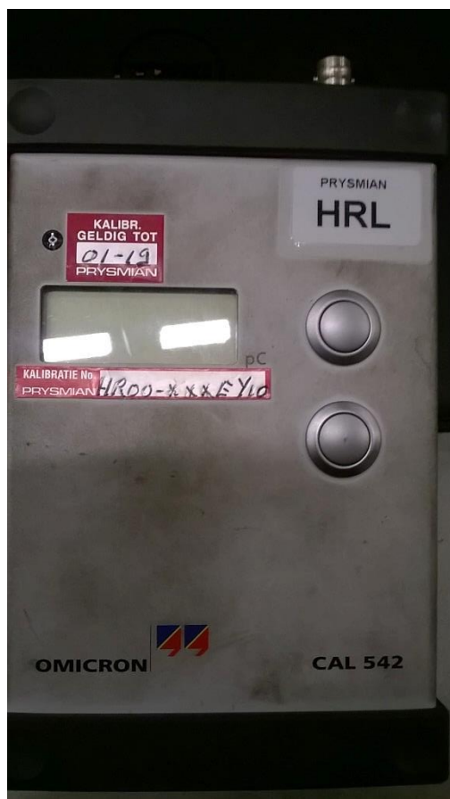
Figure 5 The PD-calibrator that was used for the tests.
